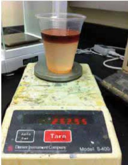
① 200g of the epoxy resin and 52g of the curing agent to the cup.
