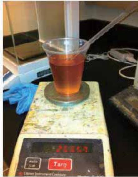
② Epoxy and curing agent is mixed well with a magnetic stir bar. Then the epoxy is degassed to remove air bubbles that can cause defects in the composite.
