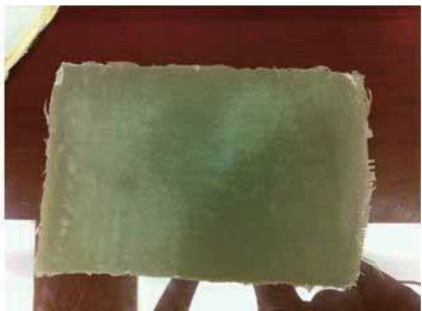
⑥ Finally the composite is hot press for 3 hours at 60°C and more 3 hours at 150°C to cure the laminates. The hot press is shown in fig. 6. After curing, take it from the bag.
