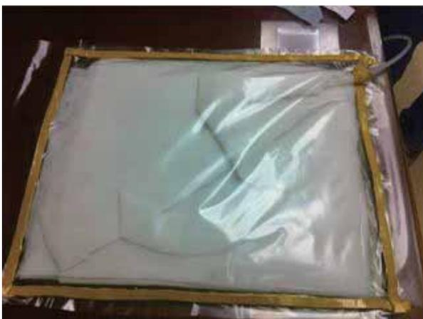
④ Vacuum bagging is used to remove excess resin. The illustration of the components of the bag is shown in Fig. 5
